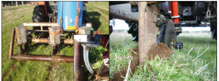
Plate 4.6: Yeomans Keyline Plow with shank pot seeders
