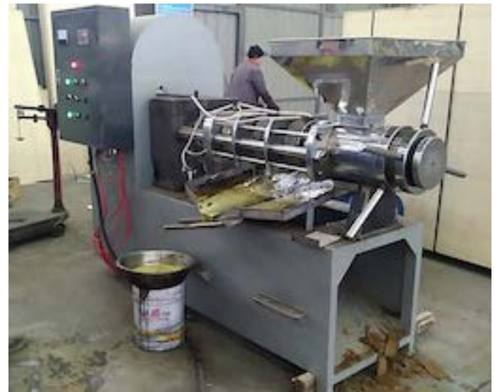
These photographs show the pressing of canola oil (rape seed oil) at two different scales. The smaller machine is suitable for many ecovillage applications
